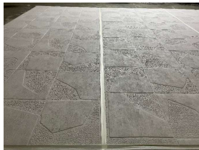
photo : detail of the joints between the multiple bands of the wall covering and the side edges, covered with a non sound absorbing tape
