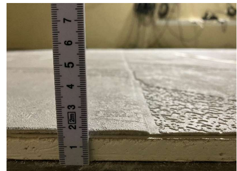
photo: cross-section of the acoustic wall cladding after bonding to BA13 plasterboard for test 2
